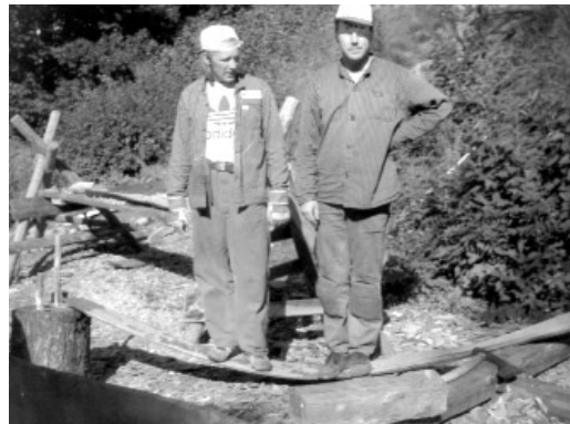
Fig. 3. The pliability of a 10–12 mm thick plank of radially split wood. Photo by the author.
