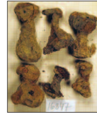
(Photo 2) Corroded clench bolts with wood residues. Trädgårdsmästaren 9–10 site. Late 11 th century.
